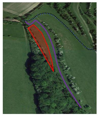
The area shown in red above is sloped and results in the most direct path (dashed line) having a cross gradient which is potentially dangerous when using a mobility scooter.
